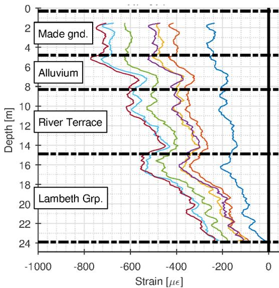
**Figure 4.** Strain change profile of a CFA pile, as it was incrementally loaded vertically in compression, with loads of 7.7 MN, 11.4 MN, 13.3 MN, 15.2 MN, 17.1 MN, 18.9 MN and 20.0 MN (corresponding to the strain profiles going from right to left). Negative strain indicates compression.
