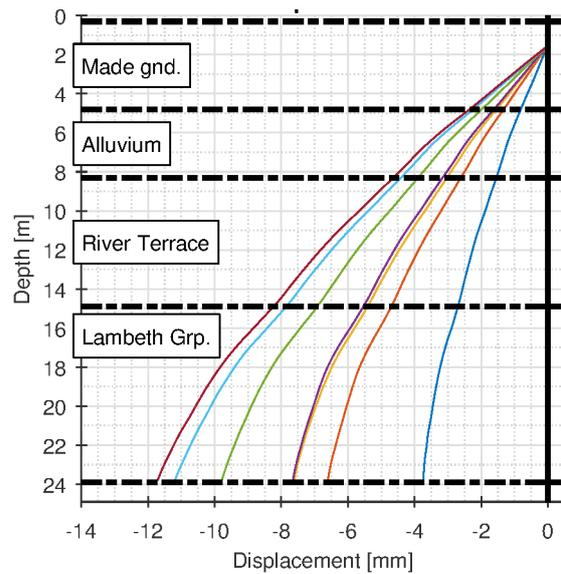
**Figure 5.** Displacement profile of a CFA pile, relative to the pile head, estimated from the recorded strain during vertical load testing as shown in Figure 4. Negative relative displacement indicates compression.
