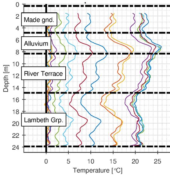
**Figure 3.** Temperature change profile of a CFA pile, recorded at hourly intervals in the centre of the pile during concrete curing, from 4 hours (baseline) to 18 hours after the pile was completed, when the concrete reached a peak temperature increase of 25.8 °C.
