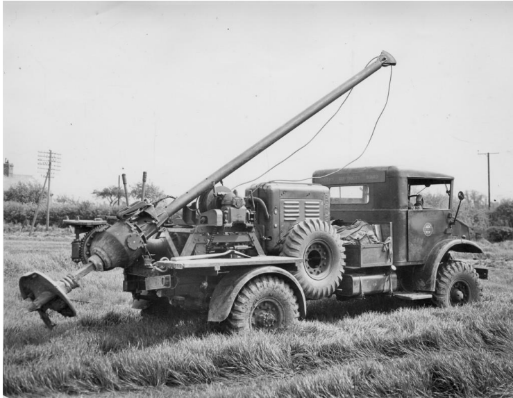
Figure 106 An ex-army vehicle for hole boring. 645
