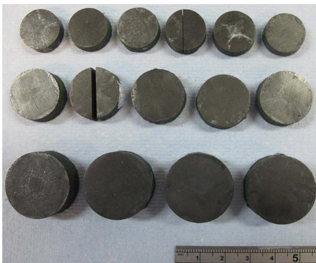
**Figure 4.** YBCO-Ag single grains of diameter (top row) 17 mm, 21 mm (middle row) and 26 mm (bottom row).
