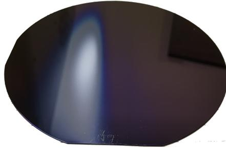
Figure 4.5: Optical Image of 4" Si wafer after 600 cycles of Alumina ALD showing a clear CVD white streak on one side of the wafer due to insufficient purging of the chamber between precursor cycles.
