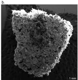
**Figure 7.** A porous version of the canola oil polysulfide. (a) Canola oil and sulfur were co-polymerised in the presence of a sodium chloride porogen. Removing the sodium chloride was achieved by soaking the milled polymer in water. The product is a sponge-like material. (b) SEM analysis of a cross-section of a particle revealed the presence of pores and channels on the order of 100–200 microns in diameter.
