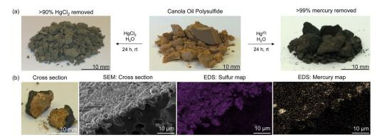
Figure 4. Mercury capture from water. (a) The canola oil polysulfide was effective in capturing both  $Hg^{2+}$  and  $Hg^{0}$  from water. The polymer changes colour to grey when it binds to  $Hg^{2+}$  and to black when it reacts with liquid  $Hg^{0}$ . (b) EDS analysis confirmed mercury was bound to the surface of the polymer.
