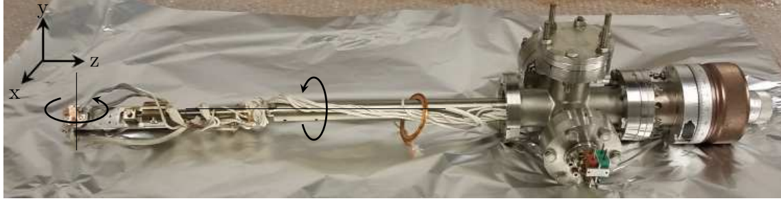
Figure 6.3: Picture of the current triple-axis manipulator, which allows for precise linear and rotational positioning of the sample within the experimental chamber with a resolution of 0.1 mm and 1^\circ . It further includes a thermocouple to measure the sample's temperature and electrical connections to measure induced currents.
