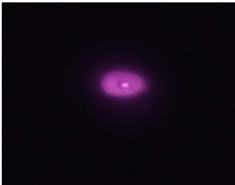
Figure A.1: A picture of spatial overlap between the probe beam (smaller stronger spot at the centre) and the THz beam, which is represented by 800 nm light surrounding the probe beam
