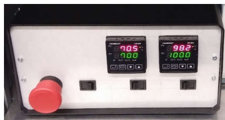
Figure 31: (left) Wiring schematic for the PID controller of the tape heater. (Right) Picture of two assembled temperature controllers panel mounted to an electrical enclosure.
