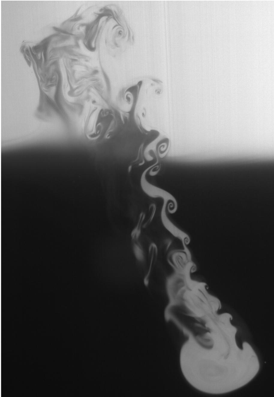
Fig. 3.12 LIF snapshot of the ring–interface interaction for  $(\text{Ri}_0, \theta_0) = (1.18, 15^\circ)$  during the transition to turbulence. The fluorescing dye clearly marks large disconnected regions of upper and lower layer fluid in the lower layer indicate significant out-of-plane motion. The instability structures in convectively unstable regions of the flow are also clearly visible, illustrating the presence of small length scales and high in-plane velocity gradients.
