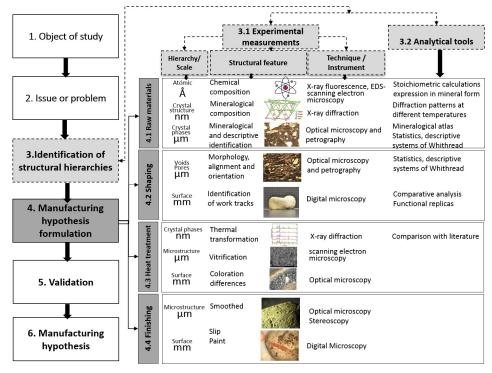
Fig 1. Methodological stages implemented to postulate the manufacturing hypotheses of the studied potsherds using a reverse engineering framework.
