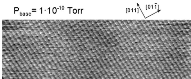
**Figure S2** Atomically resolved STM image of the Cu(100) prepared at a base pressure of  $1 \times 10^{-10}$  Torr. Imaging parameters are  $V_s=0.3$  V and  $I_t=3.6$  nA.
