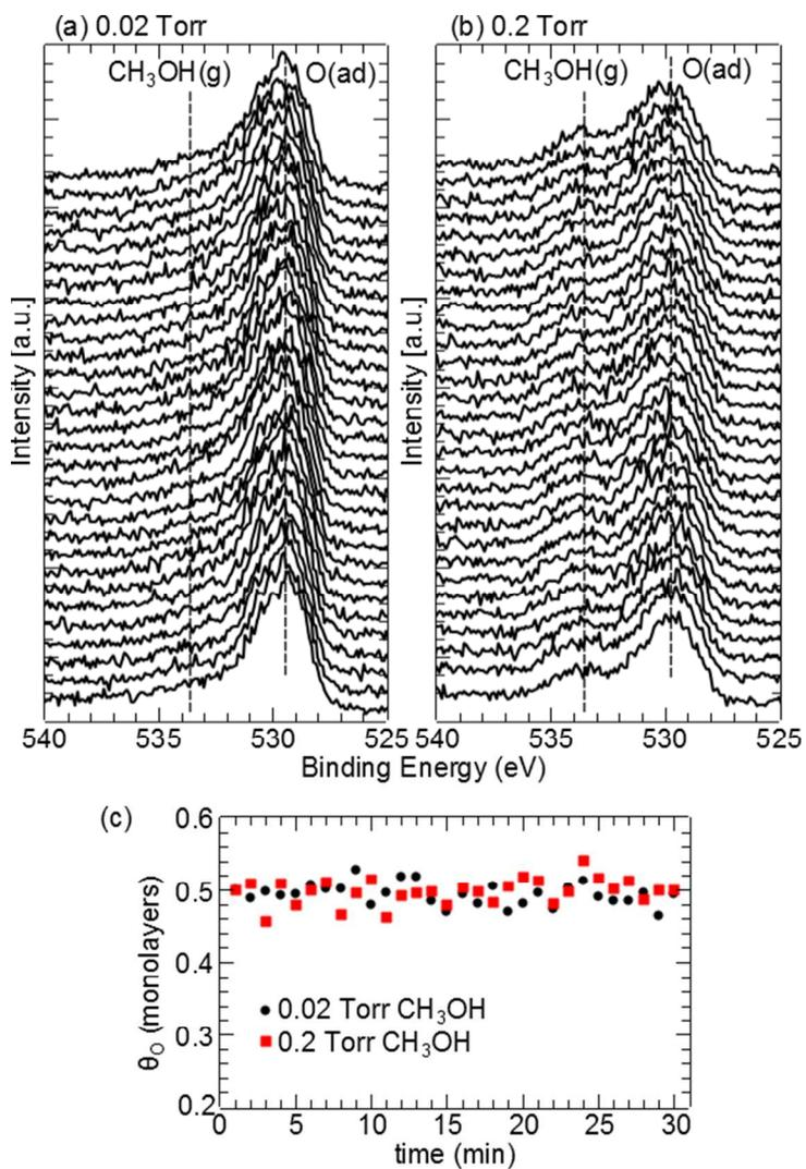
**Figure S5** O 1s region of XPS spectra of Cu(100)-(2√2×√2)R45°-O in the presence of (a) 0.02 and (b) 0.02 Torr CH<sub>3</sub>OH at 298 K, recorded at one minute intervals (upward direction for increasing duration). (c) The change in the atomic oxygen coverage over time.
