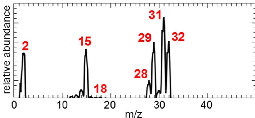
**Figure S1** Mass spectrum showing the background gas composition after methanol is dosed into the HPSTM chamber. Except for H<sub>2</sub> (mass 2), CO (mass 28) and water (masses 18 and 17) peaks, all the
