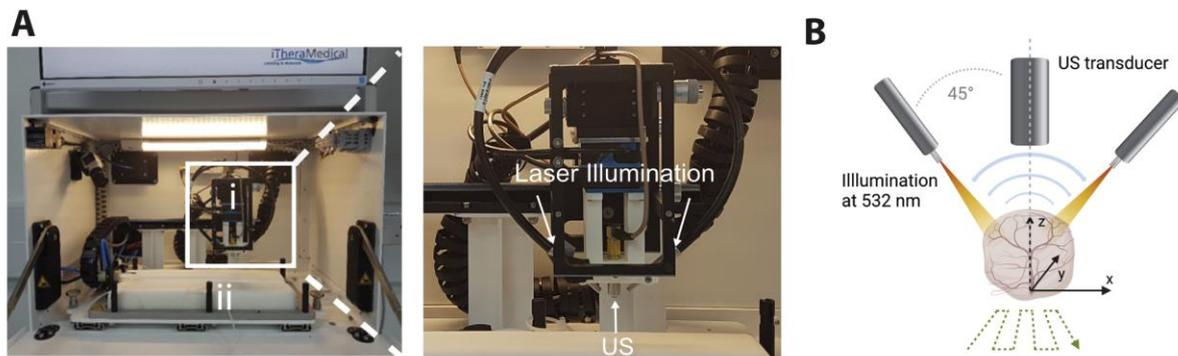
**Figure 5.2: Overview of the photoacoustic mesoscopy system.**
