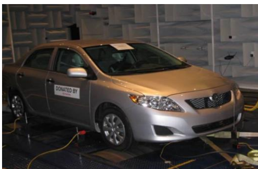
Fig. 1—Vehicle on a dynamometer in a semi-anechoic chamber for speech and noise measurements for a typical configuration; the driver was the listener and the talker was the front passenger. Separate HATS systems were used to simulate the listener and the talker.
