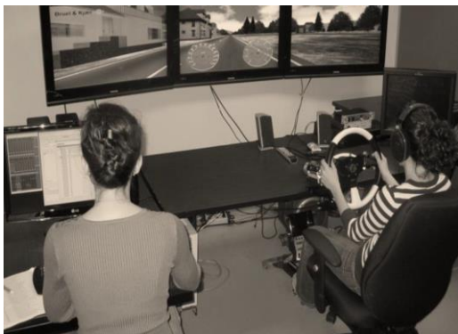
406 Fig. 2— (left) A human subject driving the simulator while listening to the HINT sentences. (right) 407 The HATS fitted with the headphones so as to check the calibration of the stimuli delivered to the listener.
