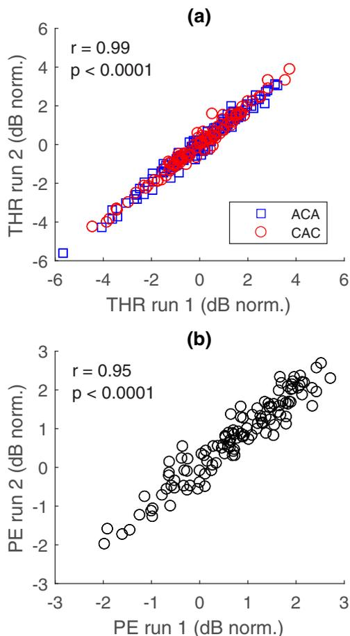
**Fig. 3.** **a** Relationship of the threshold measurements in anodic (CAC, red circles) and cathodic (ACA, blue squares) stimulation mode between the two adaptive tracks performed by all subjects. Thresholds were normalized per subject by subtracting the average threshold across electrodes from each measurement. **b** Relationship of the PE calculated separately for the two adaptive tracks
