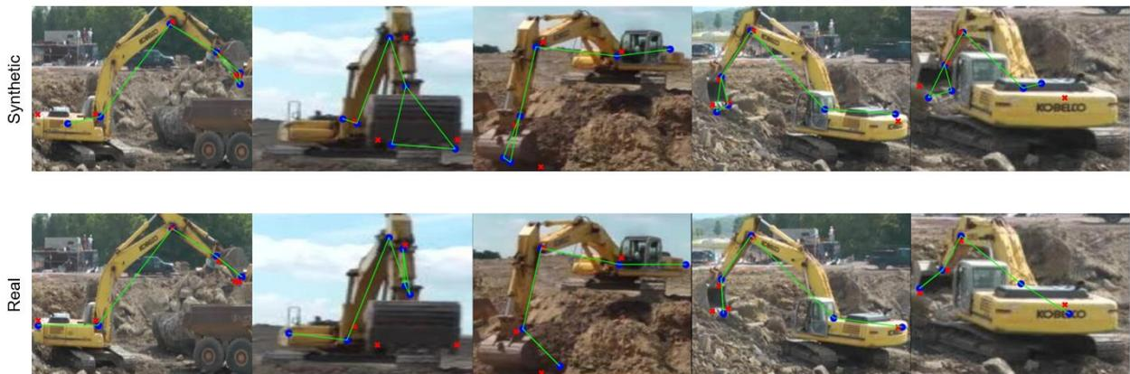
**Fig. 11.** Sample predictions for the model trained on synthetic images (top) and the model trained on real images (bottom). The predicted keypoint locations are shown with blue dots, and the ground-truth location of visible keypoints are depicted with red crosses.
