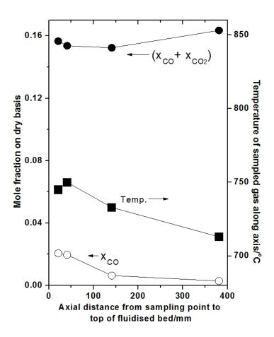
**Fig. 7.** Temperature and concentration profiles above a bed fluidised at  $750^{\circ}$ C, burning glycerol with 20% excess air ( $\theta = 0.83$ ),  $U/U_{mf} = 2.5$ , unfluidised depth of bed = 149 mm.
