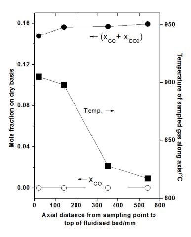
**Fig. 8.** Temperature and concentration profiles above a fluidised bed at 900°C burning glycerol with 20% excess air ( $\theta = 0.83$ ),  $U/U_{mf} = 2.5$ , unfluidised depth of bed = 149 mm.
