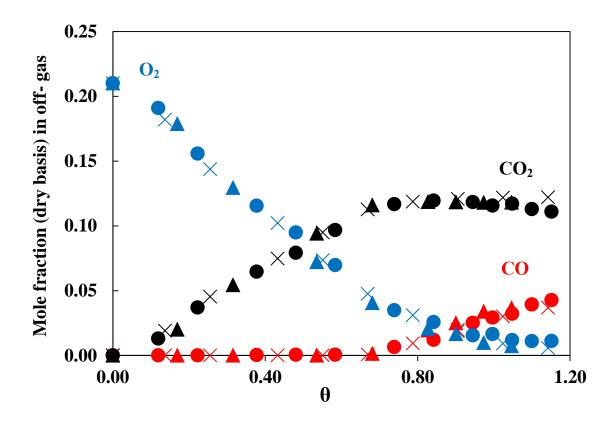
Fig. 3. Measured mole fractions of  $O_2$  (blue), CO (red) and  $CO_2$  (black) in the exhaust gas for different equivalence ratios,  $\theta$ , when burning different amounts of glycerol in air in the fluidised bed. The experiments were at : •  $700^{\circ}$ C, ×  $800^{\circ}$ C,  $\triangle$  900°C. The fluidised depth of the bed was  $\approx 175$  mm with  $(U/U_{mf}) = 2.5$ .
