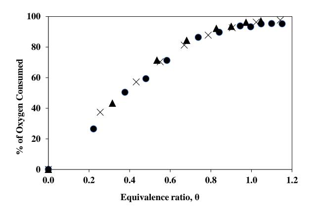
**Fig. 4.** The measured consumption of oxygen (uncertainty  $\sim 5$  %) for different equivalence ratios in a bed 162 mm deep, when unfluidised, with  $(U/U_{mf}) = 2.5$ . The temperatures were: •  $700^{\circ}$ C, ×  $800^{\circ}$ C, •  $900^{\circ}$ C.
