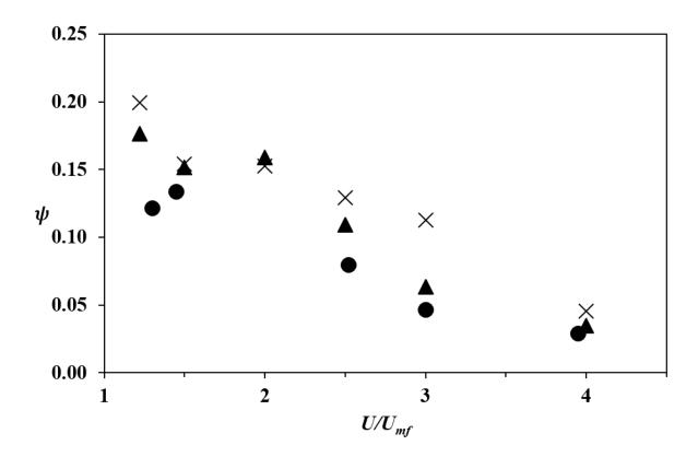
Fig. 5. The measured  $\psi = x_{\rm CO} / (x_{\rm CO} + x_{\rm CO2})$  for different  $(U/U_{mf})$  and 20 % excess air for beds 162 mm deep when not fluidised. The uncertainty in  $\psi$  was  $\sim 5$  %. The temperatures of the bed were: •  $700^{\circ}$ C, ×  $800^{\circ}$ C, •  $900^{\circ}$ C.
