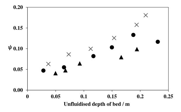
Fig. 6. The values of  $\psi = x_{\rm CO} / (x_{\rm CO} + x_{\rm CO2})$  measured for different depths of bed (when unfluidised) at  $\theta = 0.83$  and  $U/U_{mf} = 2.5$ . The temperatures were: •  $700^{\circ}$ C, ×  $800^{\circ}$ C, •  $900^{\circ}$ C.
