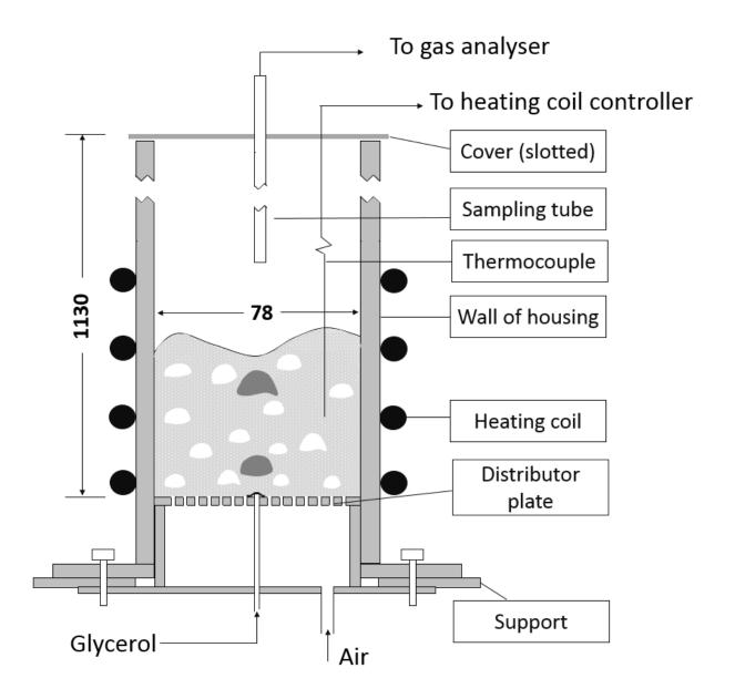
**Fig. 1.** Outline sketch (not to scale) of the electrically heated bed of alumina particles fluidised by air. Liquid glycerol was continuously pumped via a narrow tube to the centre of the distributor. The tip of the feed tube was covered by wire mesh, as shown. The tube for sampling the off-gas is also shown. Typical depths of the bed ranged from 50 to 250 mm. The central grey bubbles of glycerol vapour are surrounded by white bubbles of air. All dimensions are in mm.
