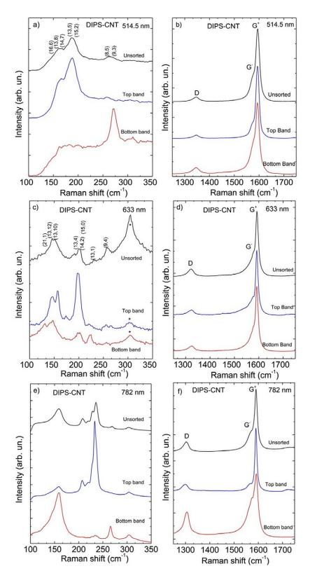
**Figure 3:** Raman spectra of DIPS SWNTs. (a) RBM and (b) G region measured at 514.5 nm, (c) RBM and (d) G region measured at 633 nm and (e) RBM and (f) G region measured at 782 nm. A peak from the Si substrate is marked with \* in (c).
