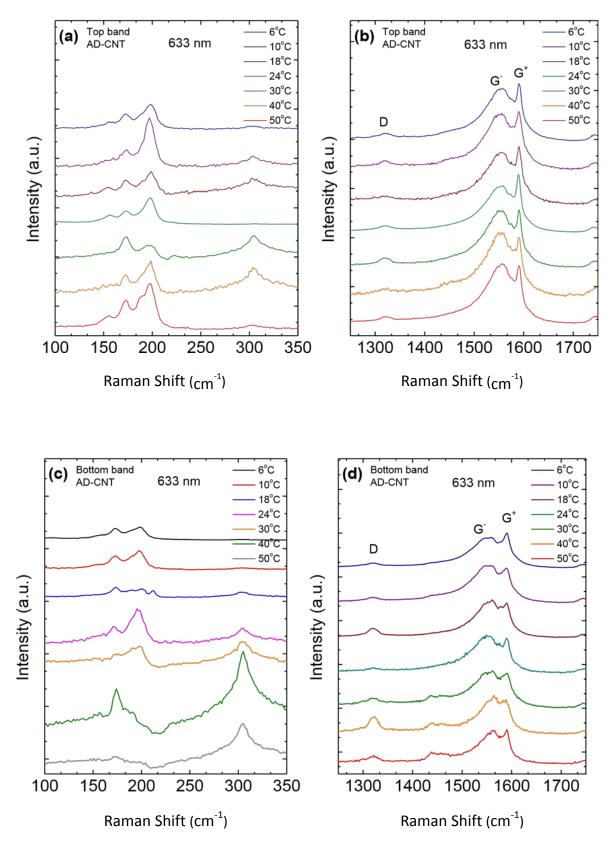
**Fig. S2.2**: Raman spectra of AD-CNTs separated at different temperatures; excitation wavelength 633 nm. (a) RBM and (b) D-G regions for top band; (c) RBM and (d) D-G regions for bottom band.
