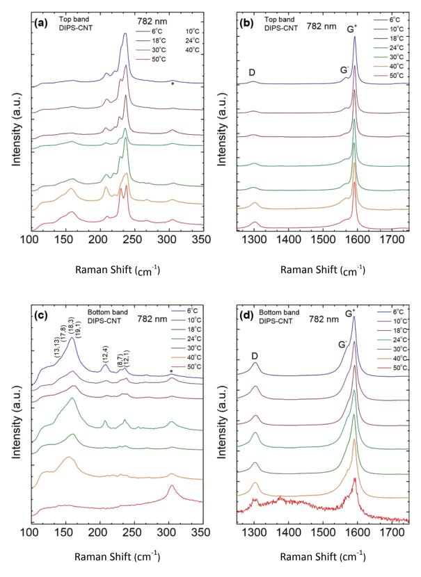
**Fig. S1.3**: Raman spectra of DIPS-CNTs separated at different temperatures; excitation wavelength 782 nm. (a) RBM and (b) D-G regions for top band; (c) RBM and (d) D-G regions for bottom band.
