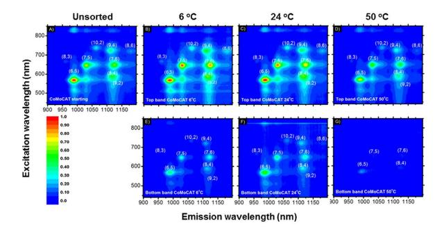
**Figure 11:** PLE maps of a) un-sorted and sorted fractions of CoMoCAT at 6, 24 and 50 °C, for b-d) top and e-g) bottom fractions. The emission intensities are normalised with the same factor used for OAS in Fig. 9b.
