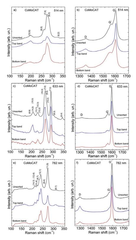
**Figure 6:** Raman spectra of CoMoCAT SWNTs. (a) RBM and (b) G region measured at 514.5 nm, (c) RBM and (d) G region at 633 nm and (e) RBM and (f) G region measured at 782 nm.
