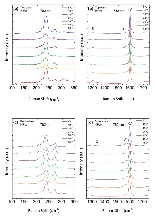
**Fig. S3.3**: Raman spectra of HiPco-SWNTs separated at different temperatures; excitation wavelength 782 nm. (a) RBM and (b) D-G regions for top band; (c) RBM and (d) D-G regions for bottom band.
