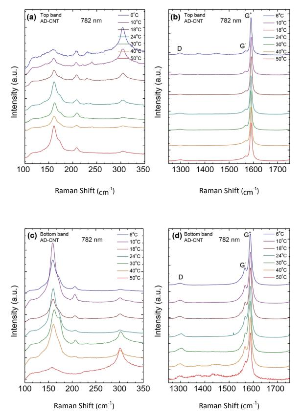
**Fig. S2.3**: Raman spectra of AD-CNTs separated at different temperatures; excitation wavelength 782 nm. (a) RBM and (b) D-G regions for top band; (c) RBM and (d) D-G regions for bottom band.
