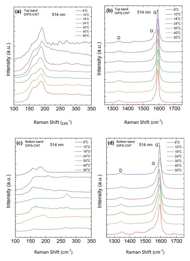
**Fig. S1.1**: Raman spectra of DIPS-CNTs separated at different temperatures; excitation wavelength 514 nm. (a) RBM and (b) D-G regions for top band; (c) RBM and (d) D-G regions for bottom band.
