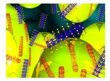
**Figure 12:** Scheme of MS-separation process. Blue tubes are m-SWNTs encapsulated with SDS forming cylindrical micelles; red tubes are s-SWNTs with low concentration of random flat SDS adsorbed on their sidewalls; textured green mass are agarose gel microbeads. The m-SWNTs remain mobile and suspended in the solvent while the s-SWNTs are physisorbed on the surface of the agarose gel microbeads.
