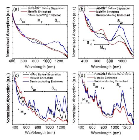
**Figure 2:** Absorption spectra of SWNTs before and after separation for (a) DIPS-CNT, (b) ADCNT, (c) HiPco, and (d) CoMoCAT. The labels  $S_{11}$ ,  $S_{22}$ ,  $S_{33}$  and  $M_{11}$  refer to the first, second, third semiconducting and the first metallic excitonic transition, respectively, and are a guide to the eye, since overlap between different excitonic transitions exists<sup>60, 61</sup>. The spectra are normalized for clear visualization.
