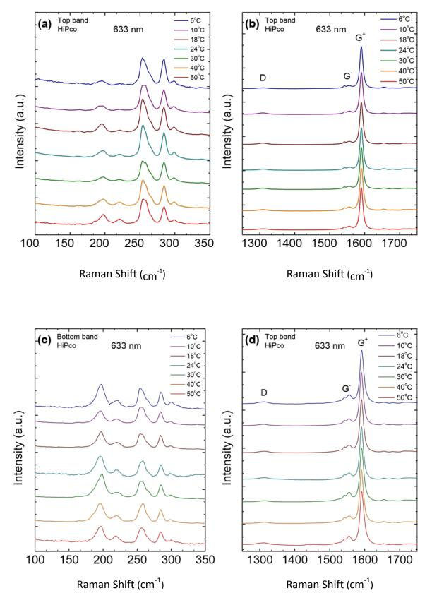
**Fig. S3.2**: Raman spectra of HiPco-SWNTs separated at different temperatures; excitation wavelength 633 nm. (a) RBM and (b) D-G regions for top band; (c) RBM and (d) D-G regions for bottom band.
