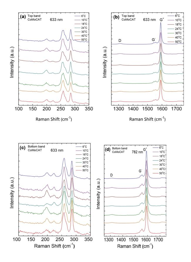
**Fig. S4.2**: Raman spectra of CoMoCAT-SWNTs separated at different temperatures; excitation wavelength 633 nm. (a) RBM and (b) D-G regions for top band; (c) RBM and (d) D-G regions for bottom band.
