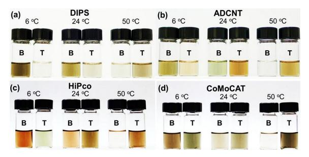
**Figure 7:** Bottom (B) and top (T) band fractions for three different process temperatures. (a) DIPS-SWNT, (b) AD-CNT, (c) HiPco, (d) CoMoCAT. The colours of the dispersions vary moving from 6 to 50 °C and for different SWNT sources.
