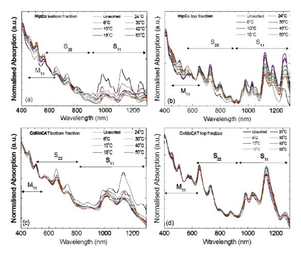
Figure 9: Optical absorption spectra for HiPco (a) bottom and (b) top band and CoMoCAT (c) bottom and (d) top band.
