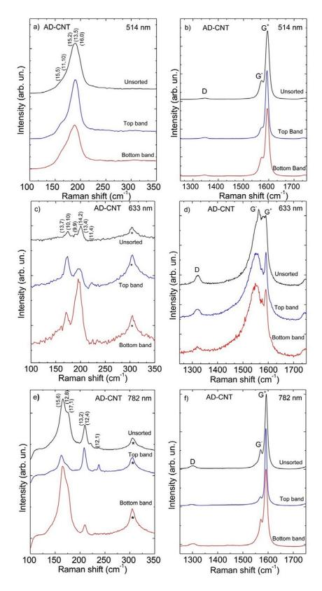
**Figure 4**: Raman spectra of AD-CNT SWNTs. (a) RBM and (b) G region measured at 514.5 nm, (c) RBM and (d) G region measured at 633 nm and (e) RBM and (f) G region measured at 782 nm. A peak from the Si substrate is marked with \*.
