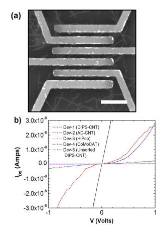
**Figure 13:** (a) SEM of representative of an array of CNT-FETs. The scale bar is 2  $\mu$ m. (b) I-V curves at zero gate bias for devices based on s-SWNTs enriched channels: DIPS-CNT (Dev-1, red), AD-CNT (Dev-2, blue), HiPco (Dev-3, magenta), CoMoCAT (Dev-4, green); and un-sorted DIPS-CNT channel (Dev-5, black).
