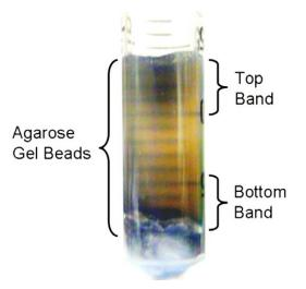
**Figure 1:** Syringe column filled with agarose gel beads. The dark colour shades are the SWNTs under separation in the column forming the top and bottom bands. The example shown here is the separation of a HiPco sample.
