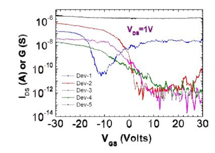
**Figure 15:** Transfer characteristics for device with sorted DIPS-CNTs channel (Dev-1), sorted AD-CNTs channel (Dev-2), sorted HiPco channel (Dev-3), sorted CoMoCAT (Dev-4) and unsorted DIPS-CNTs channel (Dev-5). The source-drain voltage, V<sub>DS</sub>, is 1 V for all curves.
