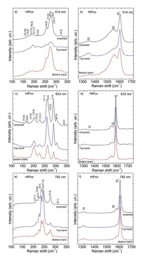
**Figure 5:** Raman spectra of HiPco SWNTs. (a) RBM and (b) G region measured at 514.5 nm, (c) RBM and (d) G region at 633 nm and (e) RBM and (f) G region measured at 782 nm.
