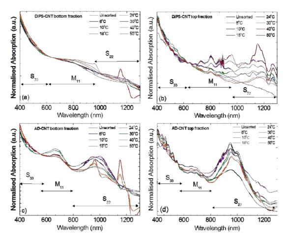
**Figure 8:** Optical absorption spectra for DIPS-CNTs (a) bottom and (b) top band, AD-CNTs (c) bottom and (d) top band. The peaks between 950 nm and 1150 nm in (b) and (d) are instrument originated noise associated with changing of source and detector.
