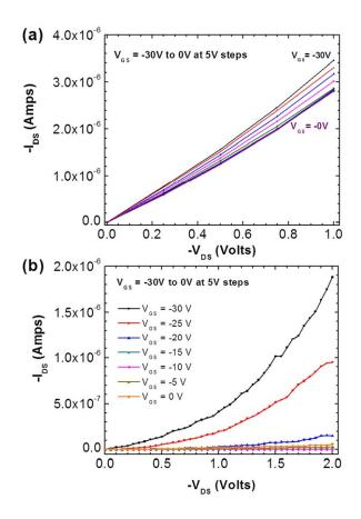
Figure 14: Output characteristics for (a) devices with un-sorted DIPS-CNTs, and (b) device with sorted DIPS-CNTs.
