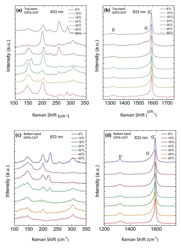
**Fig. S1.2**: Raman spectra of DIPS-CNTs separated at different temperatures; excitation wavelength 633 nm. (a) RBM and (b) D-G regions for top band; (c) RBM and (d) D-G regions for bottom band.
