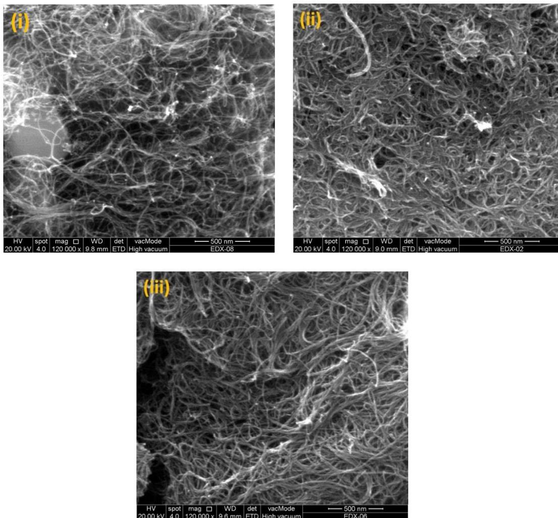
**Figure 3.** SEM images of MWCNTs samples with scale bar of 500 nm: (i) pristine MWCNTs, (ii) OD-f-MWCNTs and (iii) FD-f-MWCNTs.
