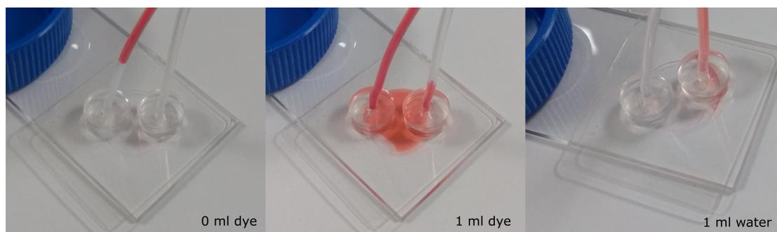
Fig. 6.8 Images of the cell used for fluorescence measurements, adhered to a glass slide rather than mica. The images from left to right show the cell filled with water, after injection of approximately 1 ml of red dye, and after subsequent injection of approximately 1 ml of water. Exchange was found to be very fast and complete. On initial filling a small air bubble was trapped, visible in the central picture to the lower left of the reservoir.
