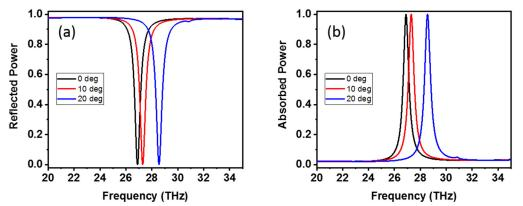
**Fig. S3:** Oblique incidence performance for TE polarization in the *xz* incidence plane. Reflection and absorption spectra for different incidence angles:  $\theta = \{0, 10, 20\}$  degrees. The performance is independent of the incidence angle. The spectral position of the absorption peak changes with incidence angle, since the magnetic field component does not remain parallel to the *x* axis.
