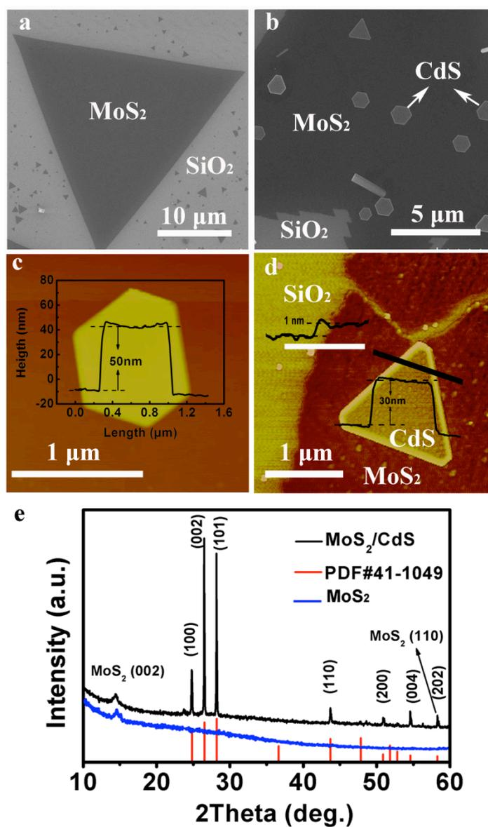
Figure 2. Characterization of vdW epitaxial CdS/MoS<sub>2</sub>. (a, b) SEM images of CVD grown triangle MoS<sub>2</sub> and CdS/MoS<sub>2</sub> heterostructures, respectively. (c) AFM image and associated height profile of a hexagonal CdS. (d) AFM phase image of the heterostructure with associated height profiles. (e) XRD characterization of MoS<sub>2</sub> and CdS/MoS<sub>2</sub>.
