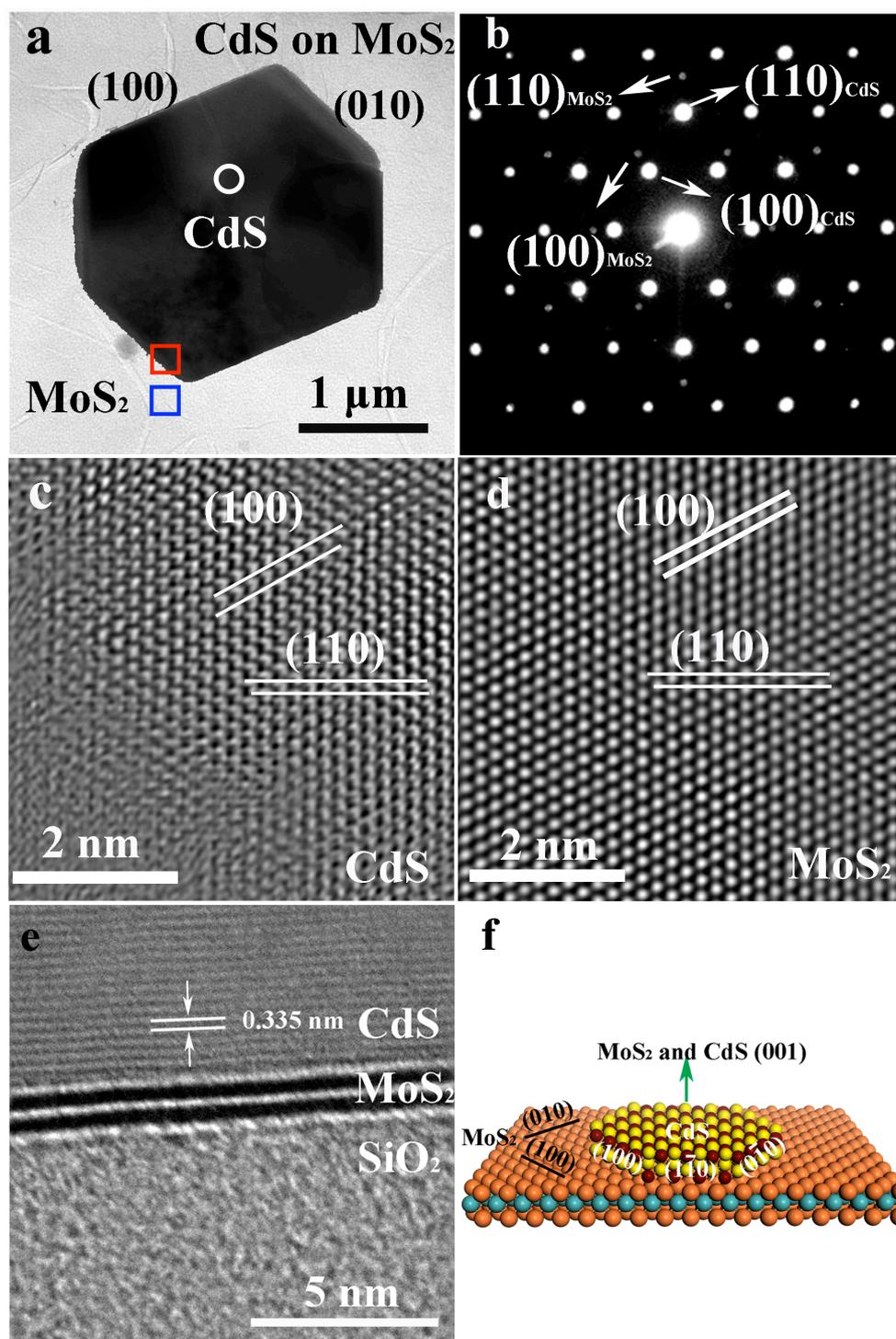
Figure 3. TEM characterization of the heterostructures. (a) Low-magnification TEM images of CdS/MoS<sub>2</sub> heterostructures. (b) Selected area electron diffraction (SEAD) of heterostructures. (c, d) Fast Fourier transform images of CdS and MoS<sub>2</sub>, respectively. (e) Cross-sectional TEM images of the CdS/MoS<sub>2</sub> heterostructure. (f) Schematic model of the CdS/MoS<sub>2</sub> heterostructures.
