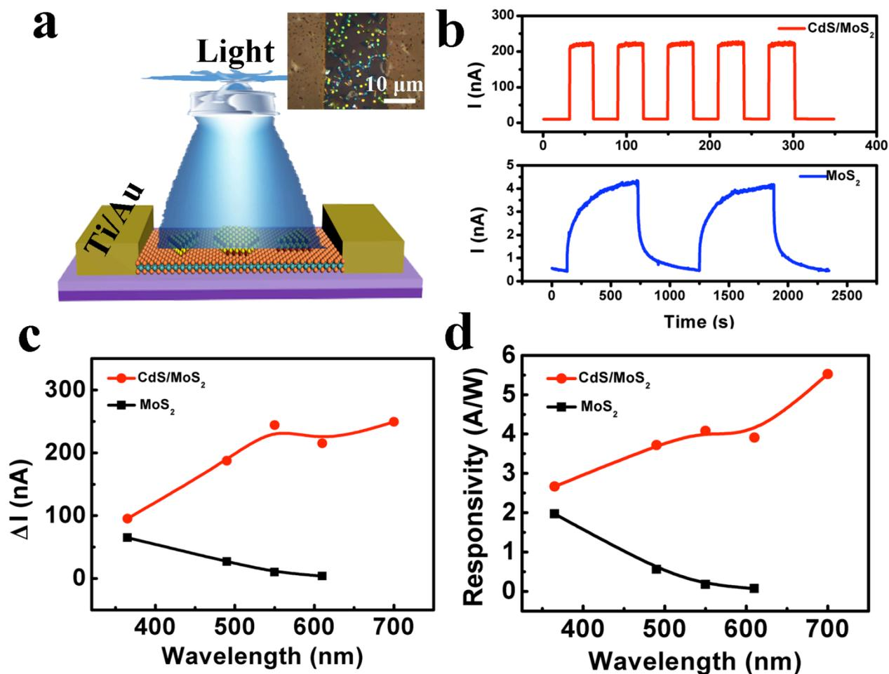
Figure 5. Characterizations of the photodetectors. (a) Schematic of CdS/MoS<sub>2</sub> heterostructure photodetector; inset shows an optical microscope image of the device. (b) Time-dependent photoresponse of CdS/MoS<sub>2</sub> heterostructure and single-layer MoS<sub>2</sub> photodetectors under 610 nm illumination, with a 1 V bias. (c, d) Photocurrent and photo-responsivity under 365, 490, 550, 610 and 700 nm wavelength of the same devices.
