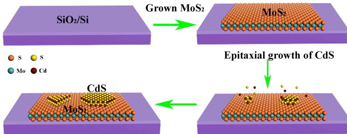
Figure 1. Schematic illustration of one-step epitaxial growth of CdS/MoS<sub>2</sub> heterostructures.
