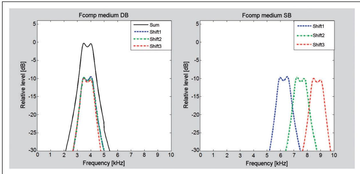
**Figure 2.** Example of the SB (right panel) and DB (left panel) for the medium setting of Fcomp. Each of the three subbands in the SB (termed “Shift1,” “Shift2,” and “Shift3” here) is transposed to the same DB. Therefore, the DB is narrower than the SB. Based on information provided by Bernafon AG.
