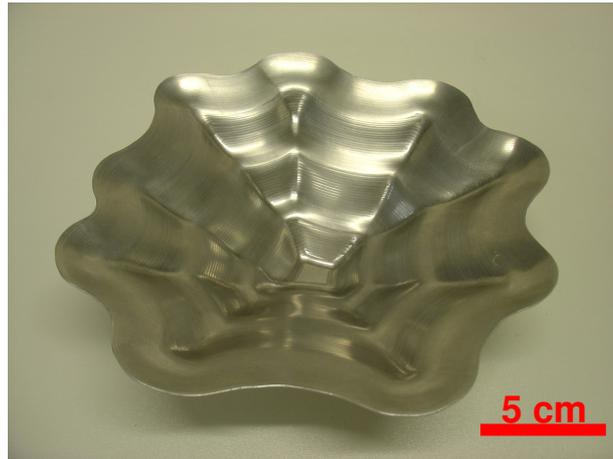
**Fig. 10.** A bespoke light shade manufactured by ISF and designed by Rachel Tomlinson, University of Cambridge in 2005. The striated surface is a desirable feature of the product.
