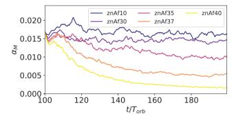
**Figure 11.** Plot showing the evolution of the Maxwell stress in simulations znAf10-40 (note that volume averages are taken over the radial range  $r = 6 - 16r_g$ ). The decreases in  $\alpha_M$  over time illustrate the weakening of MHD turbulence by eccentric disc distortion.
