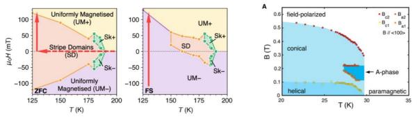
The phase diagram on the right is a typical phase diagram of bulk B20 chiral magnet MnSi [Mühlbauer et al. *Science* **323**, 915-919 (2009), which also exhibits a small skyrmion pocket (known as the A-phase) close to  $T_c$  of the material.
