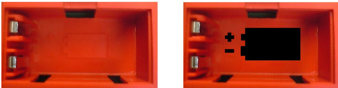
Figure 41: Although embossed, the lack of contrast affects accurate battery polarity perception
