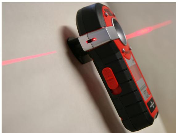
Figure 29: Black & Decker ‘Laserplus’ laser-level
