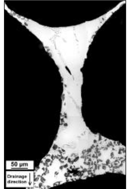
Figure 6.50: Agglomeration of SiC to form a plug at the base of a Plateau border in a carbonate based foam with  $T_{foam} = 650^{\circ}\text{C}$  and  $t_{foam} = 900$  s, cooled in air.
