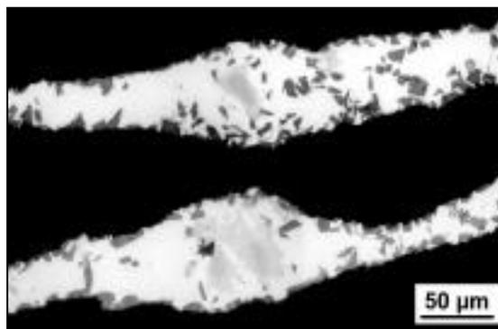
Figure 6.13:  $\text{TiH}_2$  particles embedded in a cell face (grey), surrounded by a Ti-Al compound (lighter grey)
