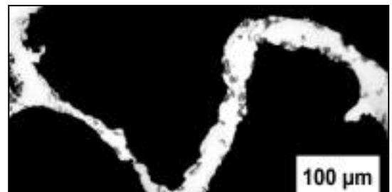
After this point brittle failure of the cell faces in the hydride-based foams means that there is no direct contact between the two sides of the band of collapsed cells. In the carbonate-based foams buckling of the cell faces continues in a uniform manner throughout the deformation process, and a physical connection between the two sides of the band of collapsed cells is always maintained.
