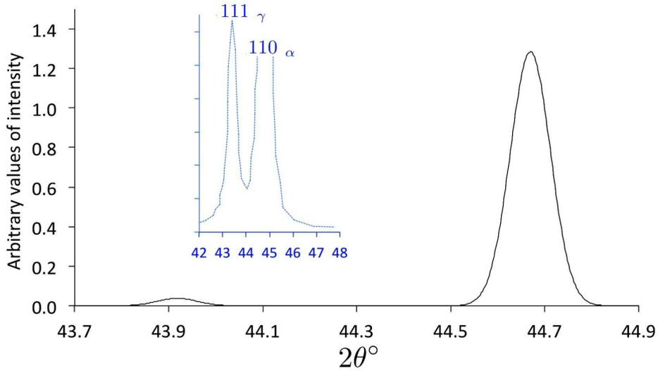
Figure 2: Simulated X-ray diffraction  $\{1\ 1\ 0\}$  pattern from a mixture of  $\alpha_b$  and  $\phi$  phases, with  $V_\phi = 0.03$ . The wavelength is 0.1541 nm,  $a_{\alpha_b} = 0.28664$  nm,  $a_\phi = 0.291$  nm. The inset shows part of an actual pattern from nanostructured bainite in order to illustrate the real breadth of measured X-ray peaks [41].
