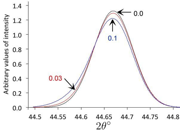
Figure 1: Simulated X-ray diffraction  $\{110\}$  patterns from a mixture of  $\alpha_b$  and  $\phi$  phases, with different  $V_\phi$  values marked on the plot. The wavelength is 0.1541 nm,  $a_{\alpha_b} = 0.28664$  nm,  $a_\phi = 0.28712$  nm, where  $a$  is the lattice parameter of the phase identified by the subscript.
