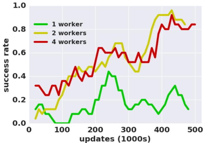
Fig. 3.7 The 7-DoF arm random target reaching with asynchronous NAF on real robots. Note that 1 worker suffers in both learning speed and final policy performance.
