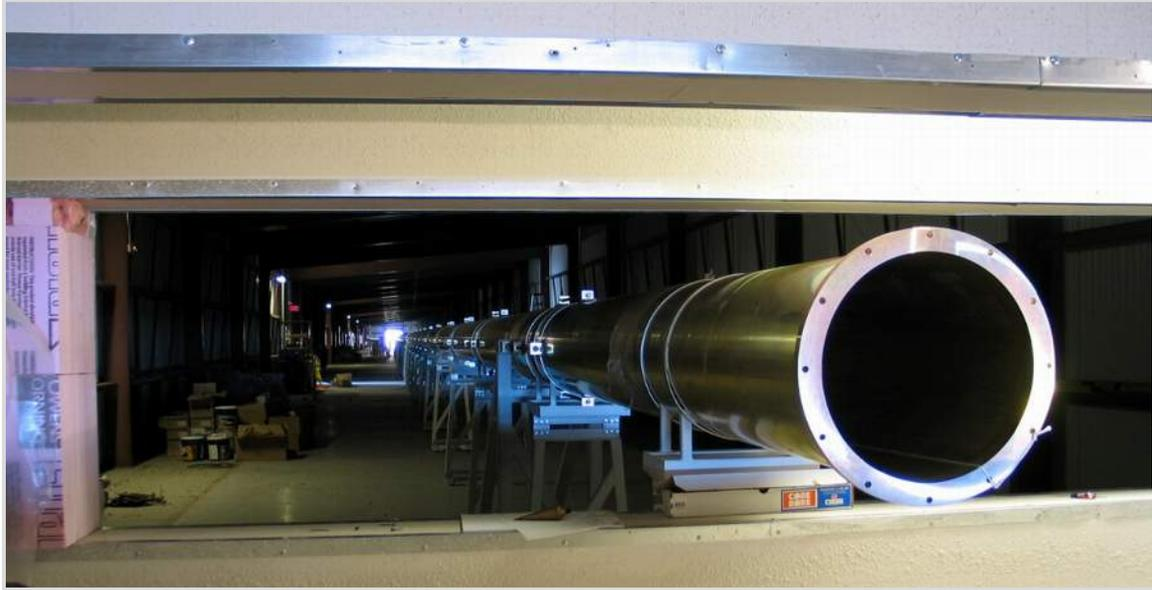
**Figure 10:** First delay line pipe installed in the delay line portion of the beam combining facility. This pipe was installed to a length of 100 meters and used for initial testing of the first delay line trolley.
