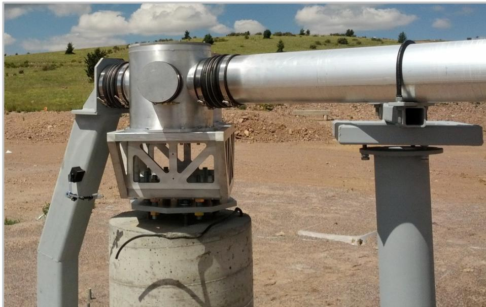
**Figure 8:** A close-up view of one of the beam relay vacuum cans mounted on its pier. This system has been designed to accept beams from the telescopes and transport them under vacuum into the beam combining facility and to the delay lines.
