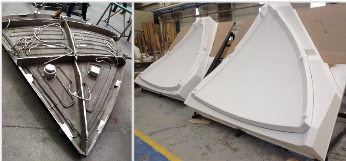
Figure 4a and b: On the left is a mold for manufacturing a portion of the MROI Unit Telescope Enclosure, and on the right are portions of the enclosure.
