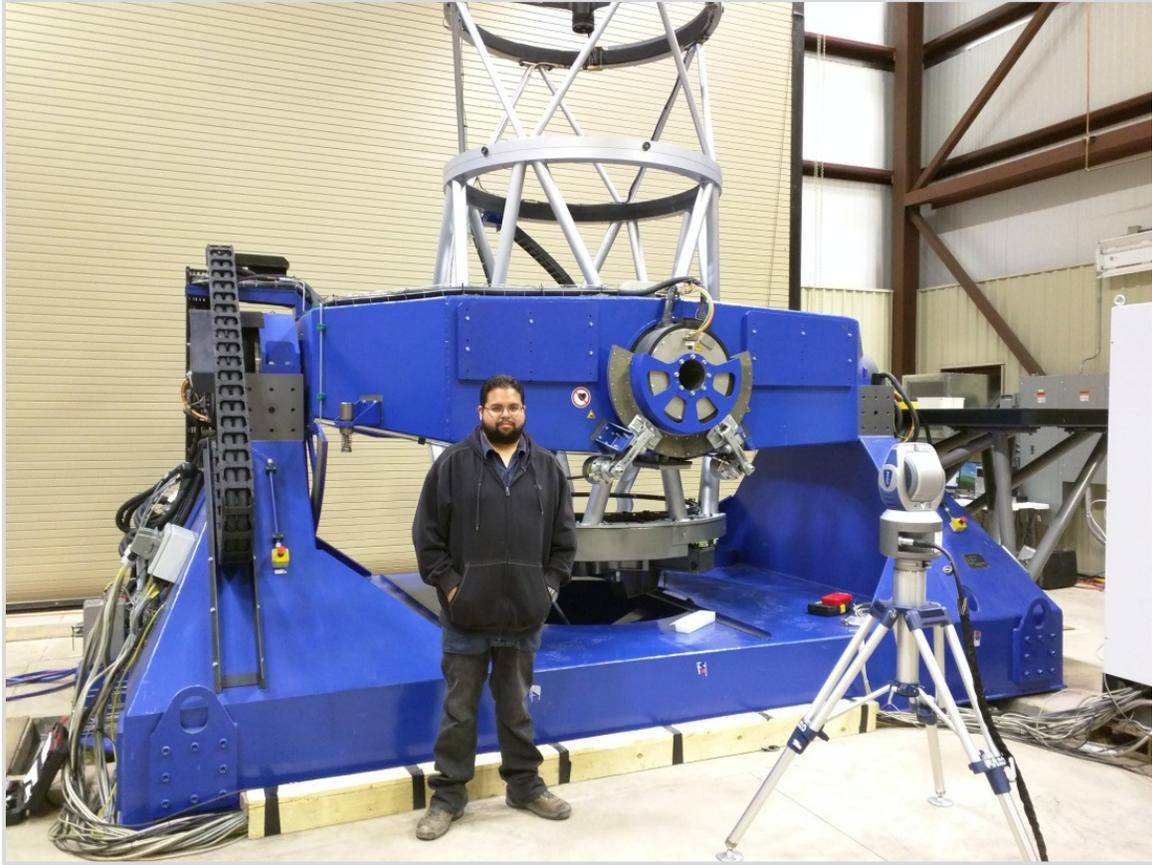
Figure 3: UTM on the kinematic mount in the VCMF. In the foreground is a laser tracking device used to align all the mirrors to the UTM structure in a few hours.
