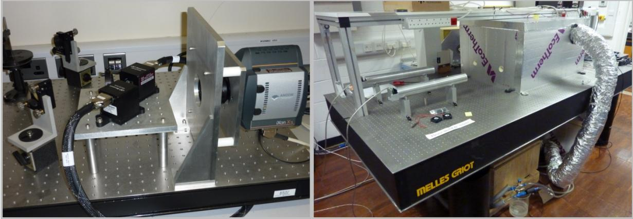
Figure 6a and b: On the left is the Fast Tip-Tilt system, specifically the FTT EMCCD, under test at Cambridge; on the right are the FTT opto-mechanics being tested (in the enclosure) with incoming fake telescope beams in a thermal enclosure to simulate performance on sky.
