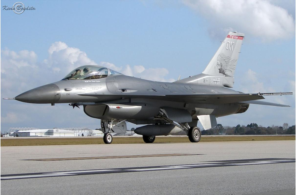
Figure 1.1: A Lockheed Martin F-16, showing its curved engine intake. Photograph by Kevin Boydston.
