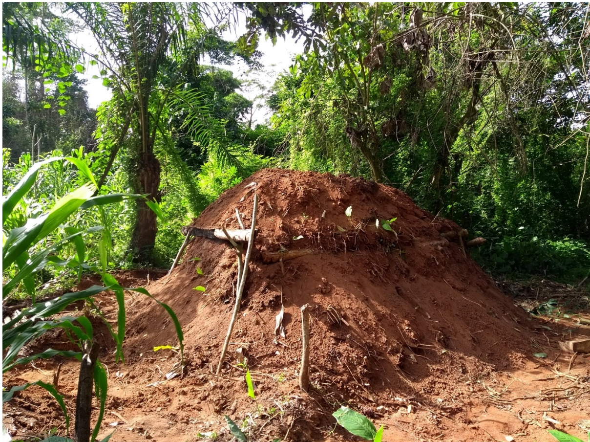
Figure 6.5 A burning charcoal mound. Wood is burning slowly beneath the soil. The mound has been fortified with branches. A ventilation hole can be seen on the shaded right-hand side. Photo taken in May 2018.
