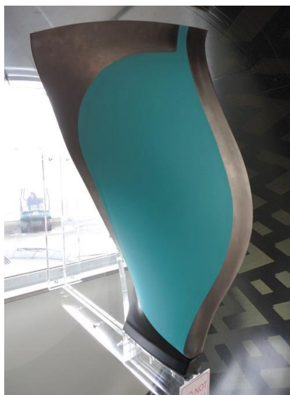
Figure 2.6 - Composite fan blade with Ti reinforcement at LE and TE (Sloan & Griffiths, 2012)
