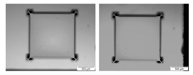
**Figure S-1.** Collection surface (*i.e.* back) of resonator (left) before collecting NaCl particles and (right) before collecting NaCl/MA particles (after using the cleaning method described by Zielinski *et al.*<sup>1</sup>). Images taken with an optical microscope (BX51, Olympus).
