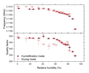
**Figure S-3.** Resonant frequencies (corrected for temperature) and quality factors for NaCl/MA mixture at each RH across both the deliquescence mode (darker, filled upwards triangles) and the efflorescence mode (lighter, open downwards triangles). Vertical error bars show the range of the five measurements with the quoted value being the average. Horizontal error bars are based on RH uncertainty ( $\pm 2\%$ ).
