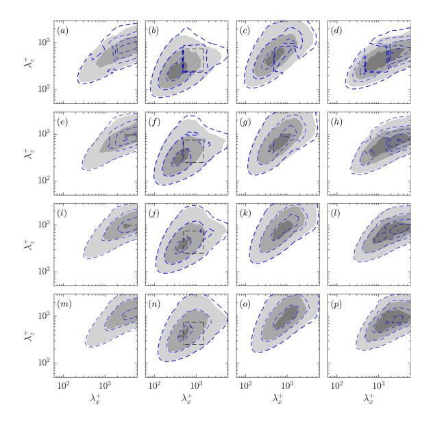
**Figure 8.** Premultiplied two-dimensional spectral densities of  $u^2$ ,  $v^2$ ,  $w^2$  and uv for case 6 (blue dashed lines) compared to the uncontrolled case (filled contours) at  $(a-d) y^+ = 173$ ,  $(e-h) y^+ = 259$ ,  $(i-l) y^+ = 350$ ,  $(m-p) y^+ = 500$ . The black dashed line encloses the wavelengths of v that are removed from the flow in the forcing region,  $y_f^+$ .
