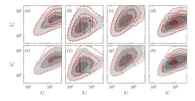
**Figure 4.** Premultiplied two-dimensional spectral densities of  $u^2$ ,  $v^2$ ,  $w^2$  and uv plotted at  $y^+ = 150$  for (a-d) cases 1 and 2 and (e-h) cases 3 and 4, and compared to the uncontrolled case at the same height. Filled contours, uncontrolled case; red lines, controlled cases. See table 1 for line styles. The black dashed line encloses the wavelengths of v that are removed from the flow in the forcing region,  $y_f^+$ .
