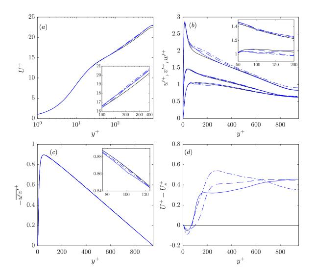
**Figure 7.** Statistics for cases at  $Re_{\tau} = 950$ , including  $\Delta U^+(y^+) = U^+ - U_s^+$ . Black lines, uncontrolled case; blue lines, controlled cases. See table 1 for line styles.
