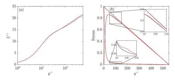
Figure 5. Additional statistics for case 1: (a) mean velocity profile for case 1 (red line) compared to uncontrolled case (black line); (b) total stress, viscous stress and Reynolds stress for case 1 (red lines) and uncontrolled case (black lines).
