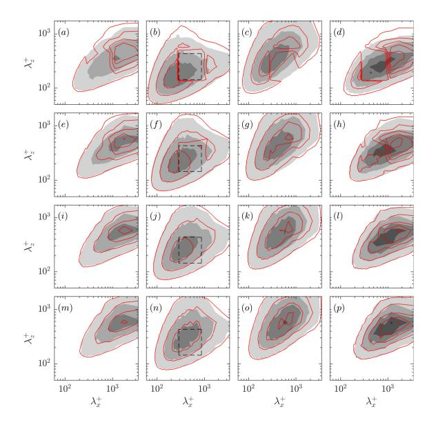
**Figure 6.** Premultiplied two-dimensional spectral densities of  $u^2$ ,  $v^2$ ,  $w^2$  and uv for case 1 (red lines) compared to the uncontrolled case (filled contours) at  $(a-d) y^+ = 100$ ,  $(e-h) y^+ = 150$ ,  $(i-l) y^+ = 200$ ,  $(m-p) y^+ = 250$ . The black dashed line encloses the wavelengths of v that are removed from the flow in the forcing region,  $y_f^+$ .
