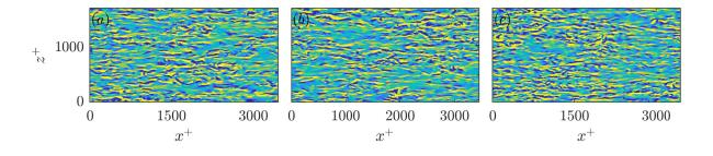
Figure 3. Instantaneous snapshots of  $v^+$  at  $y^+ = 15$  for uncontrolled case (a), case 1 (b) and case 2 (c). Blue to yellow corresponds to  $v^+ = [-0.75, 0.75]$ .
