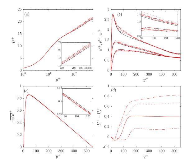
**Figure 1.** Statistics for cases at  $Re_{\tau} = 550$ , including  $\Delta U^+(y^+) = U^+ - U_s^+$ . Black lines, uncontrolled case; red lines, controlled cases. See table 1 for line styles.
