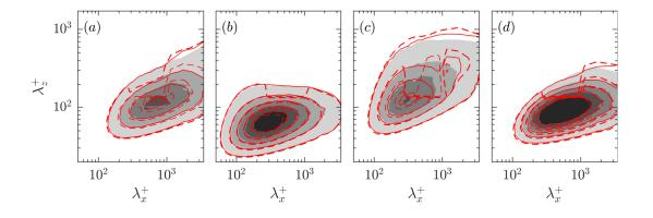
Figure 2. Premultiplied two-dimensional spectral densities of  $u^2$ ,  $v^2$ ,  $w^2$  and uv at  $y^+ = 15$  for cases 1 and 2 (red lines) compared to uncontrolled case at the same height (filled contours). See table 1 for line styles.
